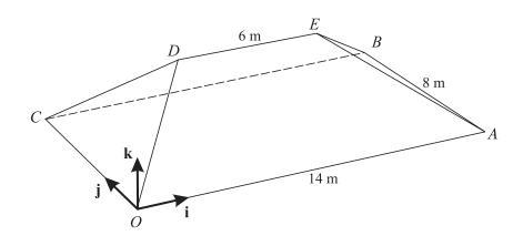
The diagram shows the roof of a house. The base of the roof, OABC, is rectangular and horizontal with  $OA = CB = 14 \,\text{m}$  and  $OC = AB = 8 \,\text{m}$ . The top of the roof DE is 5 m above the base and  $DE = 6 \,\text{m}$ . The sloping edges OD, CD, AE and BE are all equal in length.
